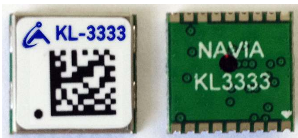
Fig. 3. The exterior of the receiver NAVIA GNSS - KL 3333 top and bottom view (not in scale 1:1).
