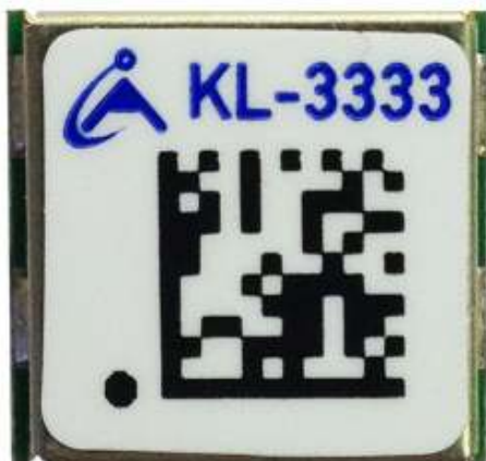
Fig. 2. The exterior of the navigation receiver NAVIA GNSS - KL 3333 (Not to scale 1:1)
